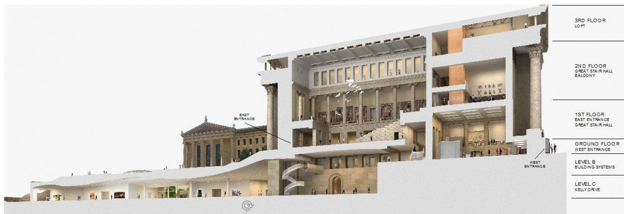
Rendering of the Museum's six floors. The scope of work of the Core Project will take place on Levels A, B and C. Level C has been closed to the public for decades and will be reopened as part of the Core Project. Level B houses the Museum's systems.
